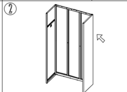
Bolt the right side with back plate. In the same way as the first step
